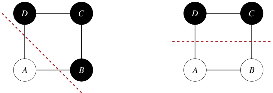
Figure 12.12: Two cuts of a graph with four vertices and four edges
