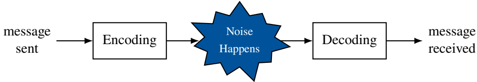
Figure 6.1: The process of sending information on a noisy channel
